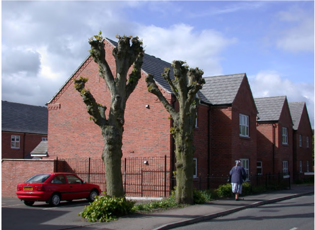
Figure RT6 Building so close to retained trees leads to problems with shade and leaf litter. This can result in trees being mutilated and high future maintenance costs.
