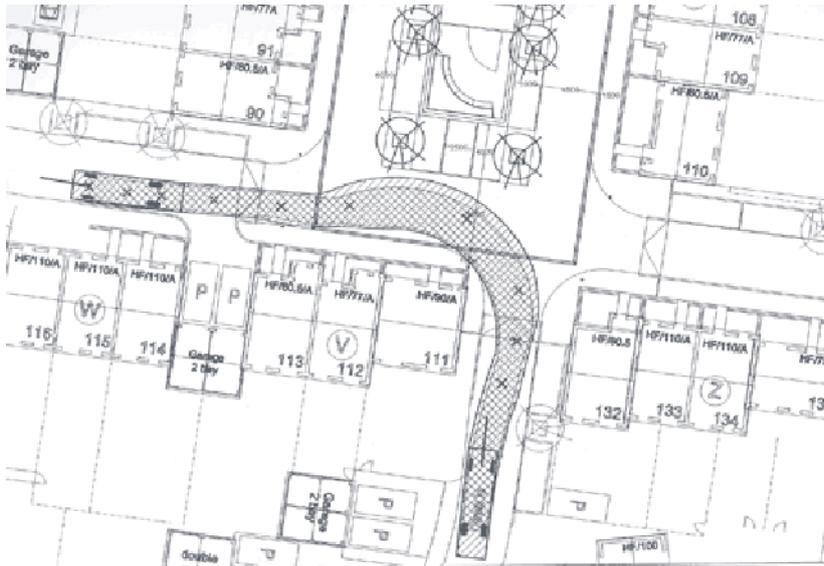
**Figure GL4 Example of tracking. (Reproduced with kind permission of Jelson Ltd and Boreham Consulting Engineers.)**
